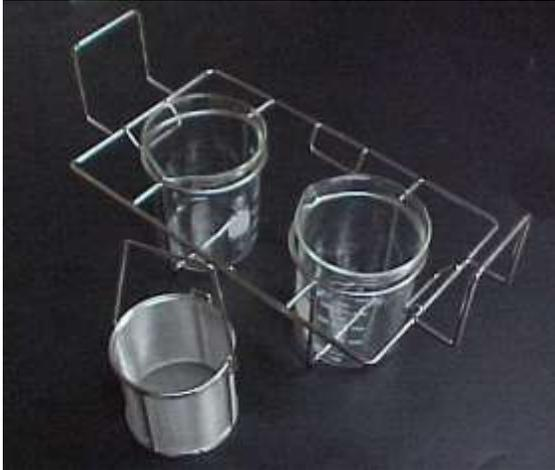
9. Some very small parts are better cleaned in a Pyrex beaker. The beaker should be suspended in the ultrasonic tank using a beaker holder. This positions the beaker for maximum effectiveness in cleaning.
