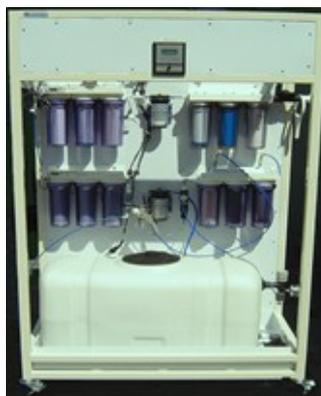
Larger Lab systems up to 500 gallons per day are available; these systems will provide water enough for limited production cleaning of parts. They can also be designed to supply 4-5 stations within a lab to provide water to faucets or other equipment on demand. These Systems can be remote controlled by having the control panel in the lab and the DI unit in another room.
